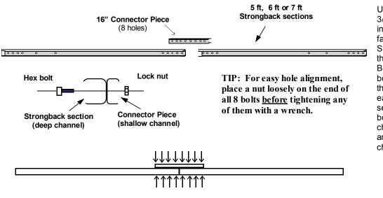
Using the bag of (8) ea 3/4" hex bolts and nyloninsert lock nuts, secure fasten the two sections of Strongback together with the 16" connector piece. Be sure to use all eight bolts and nuts, fastening through the first 4 holes on each of the Strongback sections. Be sure the bolts are in the Strongback channel, and the lock nuts are in the Connector piece channel, as shown.
