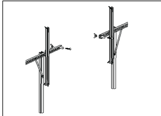
FIG 8A—Place Center Stops in 1st hole on each base frame as shown, using bolt, wing nut and plastic sleeve. (View is from front of frame).
