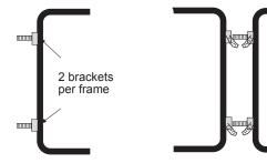
Double displays thread through brackets on both frames as shown.
