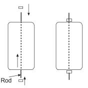
Holding the bottom collar on the rod, lift the panel and insert the top of the rod into the thru-hole in the Top Arm. Push it as high as it will go. The bottom of the rod will just barely clear the bottom Arm. Maneuver the bottom of the rod into the hole in the bottom Arm.
