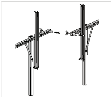
FIG 7A —Place Center Stops in 1st hole on each base frame as shown, using bolt, wing nut and plastic sleeve. (View is from front of frame).
