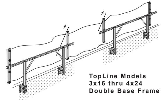
The banner installs on all TopLine Models by turning the End arms - with the banner attached - inward and sliding them onto the Strongback. If your model has one or more Center Arms, you will need to locate the Retaining Rod(s) on the outside of the banner. When properly installed, the banner wraps around and conceals the End arms - if the banner does not conceal the End Arms it is not installed properly and wind damage can result to your banner and framework.
