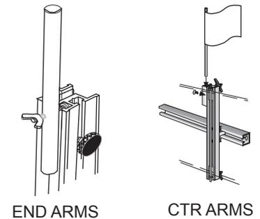
If not already done, screw the 3" Lock Knob into the Glide on the Dead End Arm. Pull the Arm outward until the banner is as tight as you can get it. Tighten the Lock Knob to hold the Arm in place.
