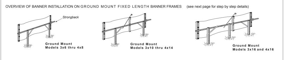
The banner installs on all Ground Mount Models by turning the End arms - with the banner attached - inward and sliding them onto the Strongback. If your model has one or more Center Arms, you will need to locate the Retaining Rod(s) on the outside of the banner. When properly installed, the banner wraps around and conceals the End arms - if the banner does not conceal the End Arms it is not installed properly and wind damage can result to your banner and framework.
