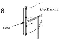
Pull the Live End Arm across the frame to the left side. Turn the Live End Arm inward so its glide can insert into the Strongback. Insert it and slide it in until it hits the white plastic Stop.
