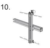
After the banner is fully taut, tighten the knobs at the top & bottom of the Center Arm(s), pulling the Retaining Rod(s) tight against the front of the banner.
