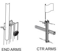
Add the Accent Flags to the Arms as shown. For End Arms, insert bolt into channel on side of arm and tighten wing nut. For Center Arms, drop into channel and tighten thumbscew
