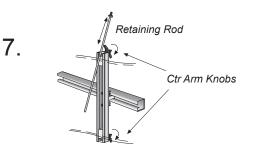
If your model has one or more Center arms, loosen the black knobs at the top and bottom and slide the Retaining Rod high enough to place it over the front of the banner. Re-insert the Rod through the bottom eyelet, but do not re-tighten the knobs yet.
