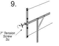
If not already done, insert the 7" Tension Screw into the threaded hole in the Glide in the Live End Arm until it hits the white plastic Stop. Continue to wind until the banner becomes fully taut. The banner should be straight across the top.
