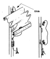
Squeeze a dab of grease onto 1-2" of the tip end of the **Tension Screw**.
